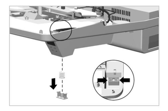
Figure 6-30. Removing the Monitor Support Cover Cap Reverse the above procedure to install the monitor support cover cap.
